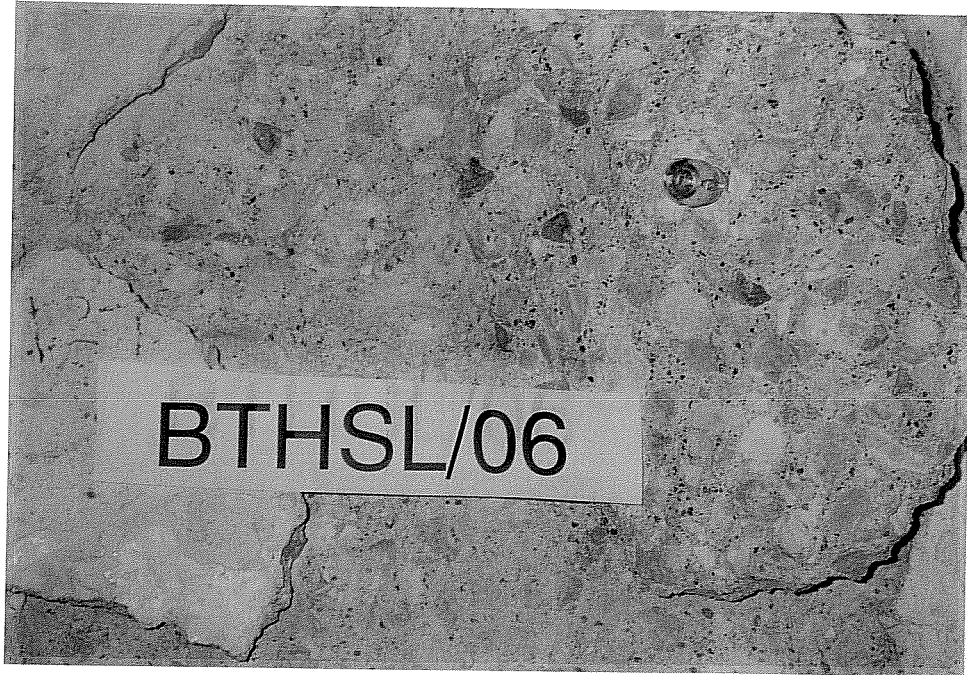
Figure 5.9 Tensile baseline expansion anchor concrete cone breakout
