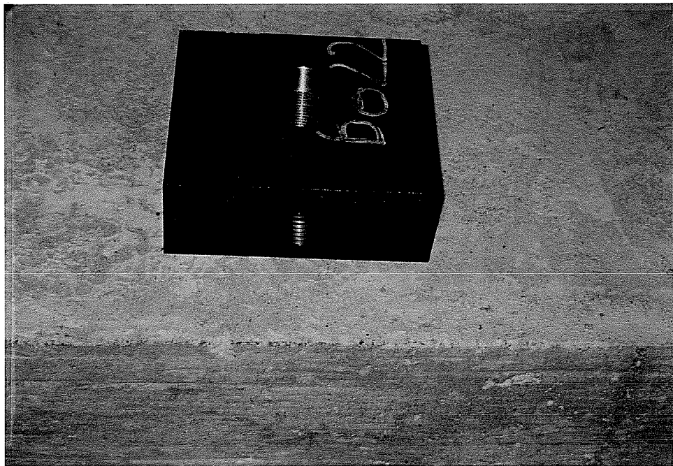
Figure 4.10 Typical shear loading plate
