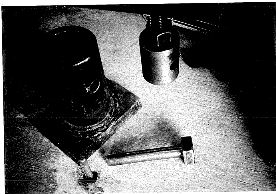
Figure 4.6 Typical baseline tensile loading shoe
