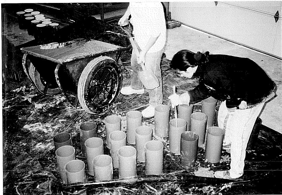
Figure 4.5 Casting concrete test cylinders
